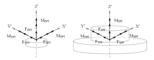
Figure 3-1. 3-dimensional force components at tower top and foundation
